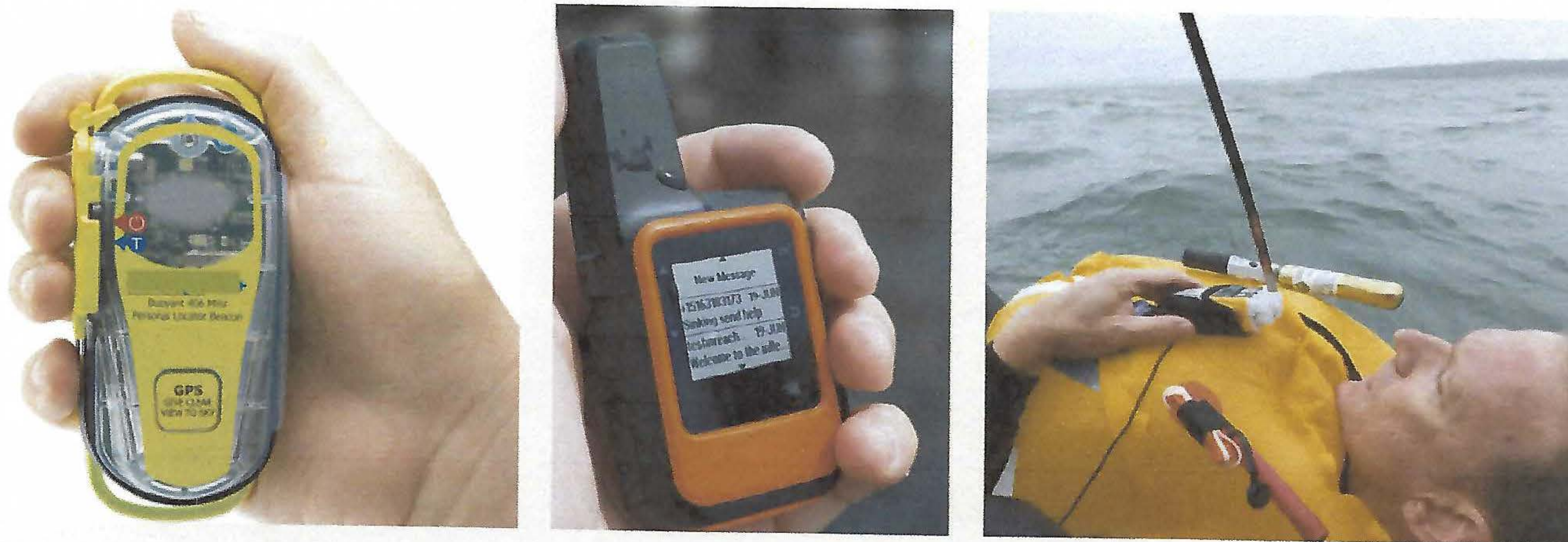
Figure 1. Exemplar PLB (left) and SEND (center), and PLB attached to lifejacket (right).
